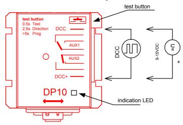
For the purposes of DP switch function testing, a DC power supply of 9-16V, with marked polarity, can also be used. Only for functional test, by button.
